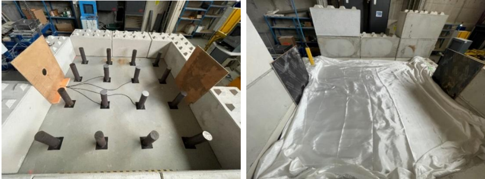
Fig. 2. The configuration of the laboratory tests and installation of the geotextile.
