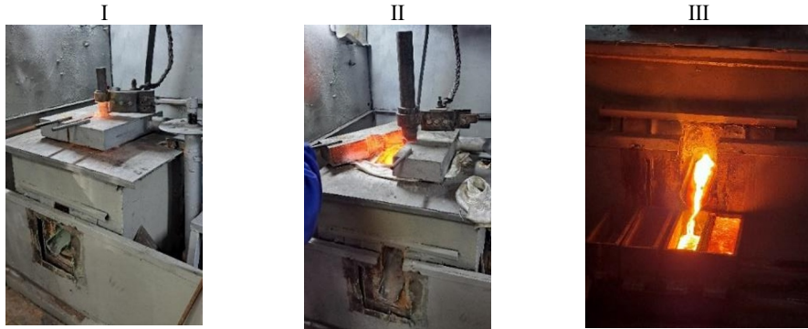
I- furnace ignition, II – melting, III – draining the melt
