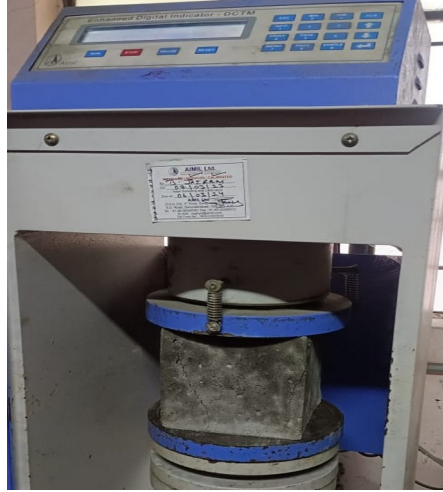
Fig.2. Cube test in Compression Testing Machine
