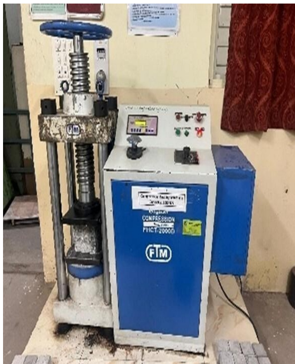
Figure 5: Compressive Strength Test (UTM)
