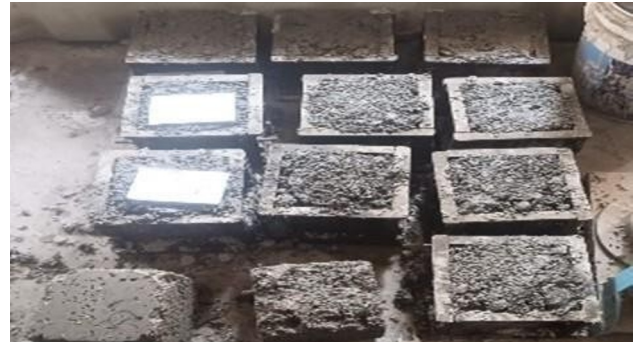
Figure 4: Concrete placed into cube moulds
