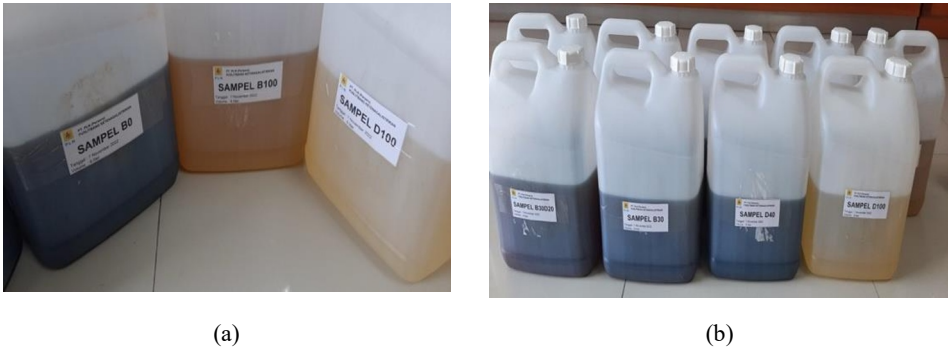
Fig. 1. Physical appearance of fuel samples (a) pure petrodiesel (B0), pure FAME biodiesel (B100), and pure HVO (D100) (b) Mixture of petrodiesel, FAME biodiesel, and HVO.
