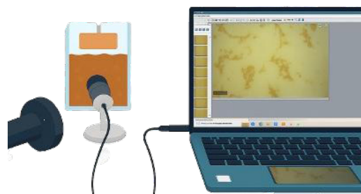
Fig 1. Systematics of floc imagery using digital microscopes
