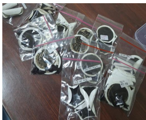
Fig 13. Sludge obtained at the optimum dosage analyzed using SEM-EDX and FTIR
