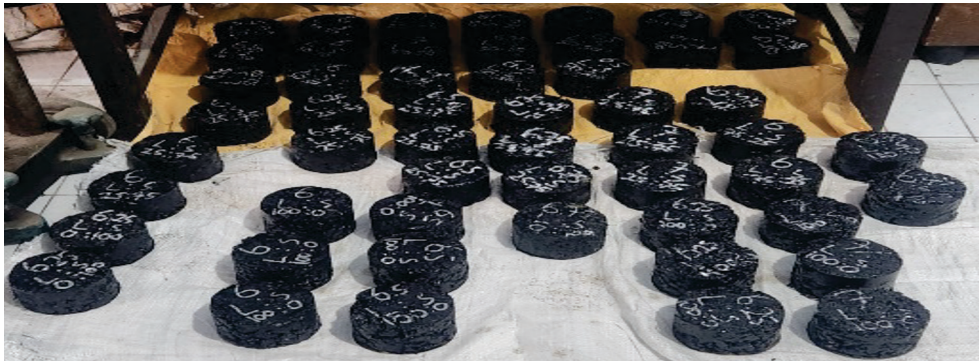
Fig. 2. Test Specimen of Stone Matrix Asphalt Mixture
