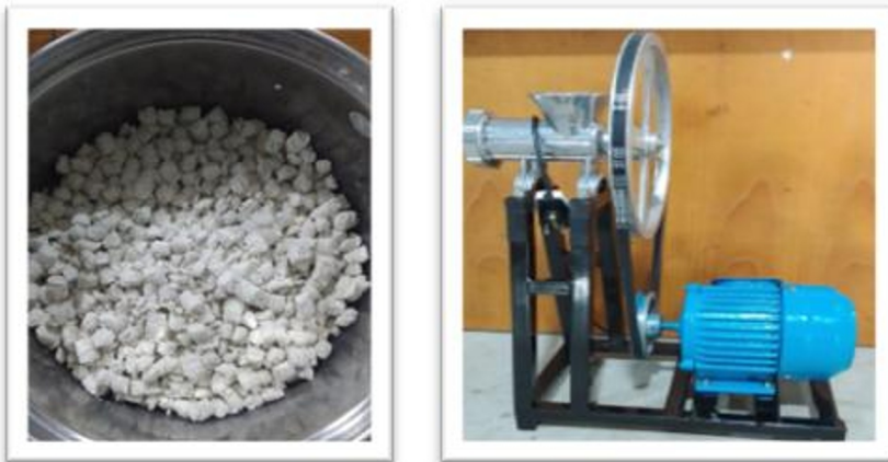
Fig. 3. Catfish pellets are produced by automated pellet feed production machines
