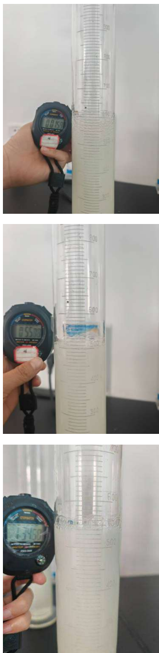
Fig. 4 Defoaming of fracturing fluid with alkyl polyglycosides by polyether-modified organosilicones and polyether antifoam agents
