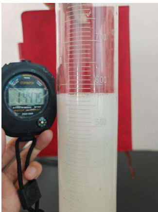
Fig.3 Defoaming of fracking fluid with betaine surface activator by polyether-modified organosilicone and polyether defoamer
