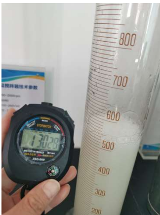
Fig. 2 Defoaming of secondary modified guanidine gum fracturing fluid by polyether-modified organosilicones and polyether defoamers
