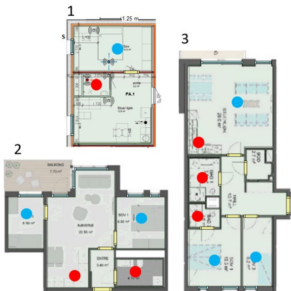
Fig. 1. The 3 apartments that were modelled and investigated in this study. Apt 1: 30 m 2 , Apt 2: 47.5 m 2 , Apt 3: 71 m 2 . The blue dots indicate the placement of supply vents, while the red dots indicate extract vents.
