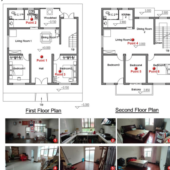
Fig. 1. Distribution diagram of indoor thermal environment measuring points.
