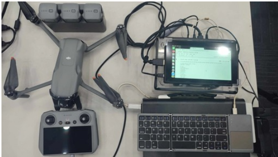
Fig. 5. Hardware setup including drone, microcontroller, and display unit.
