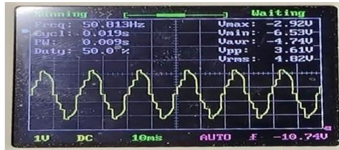
Fig. 6. The output obtained in CRO with RL Load.
