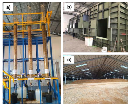
Fig. 3. The Nickel Heap Leaching Test Stages from a) Column Test, b) Crib and c) Cell Sized Test
