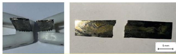
Fig 8. Bending test result on Cu-27.66Al-12.39Mn alloy after quenched with DQ method
