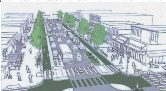
Fig 3. Example of reconstructing a transport-pedestrian street with a reduced width of the roadway to "calm" traffic movement: a - Street view before reconstruction; b - Street view after reconstruction.
