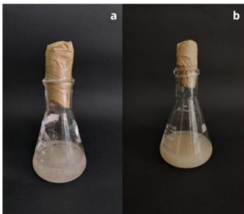
Fig 3. The keratinase production medium prepared using submerged fermentation (SmF) with chicken feathers as the sole carbon and nitrogen source (a), the medium after three days of fermentation by Bacillus sp. MD24 (b).
