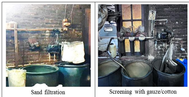
Fig.3. Filtration process of ciu bekonang.
