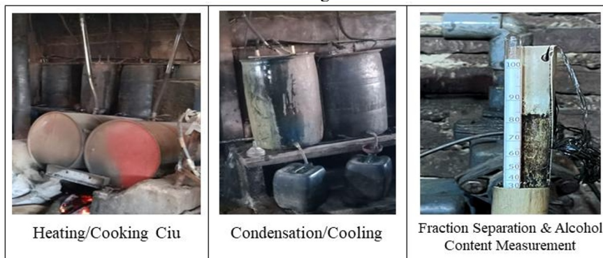
Fig.2. Distillation technology process of ciu bekonang.
