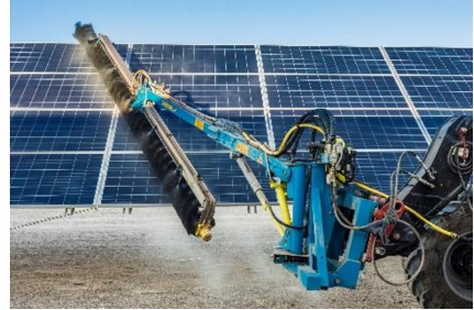
Fig. 8. Mechanized cleaning of photovoltaic modules.
