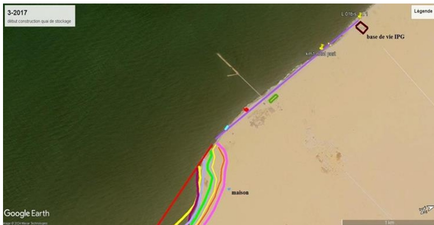
Figure 3: The pier length estimated at 850 m; slight sediment accumulation observed north of the port
