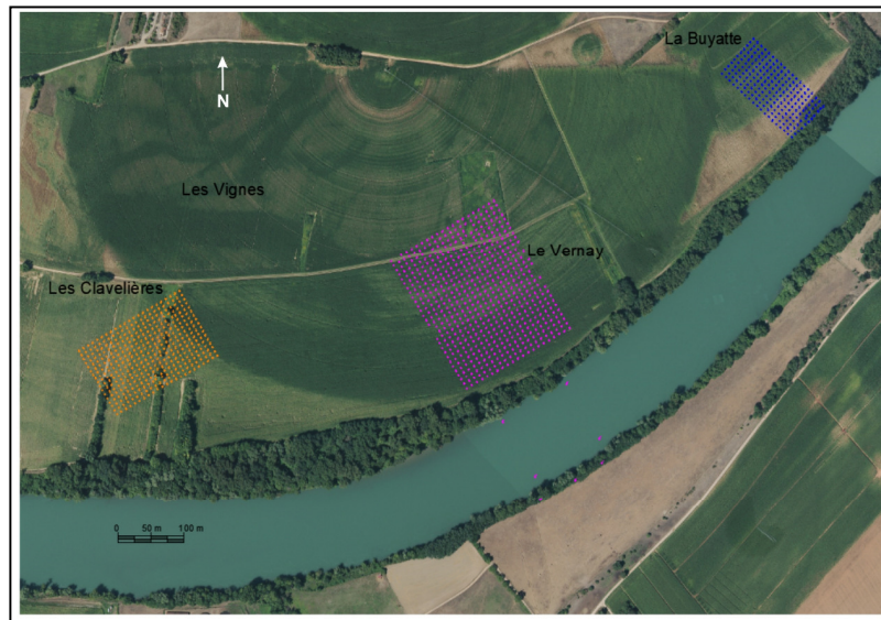
Fig. 1. Sensor networks including underwater nodes in the Rhône River. Yellow dots : 391 nodes in the Clavières site, purple dots : 604 nodes in the Vernay site, blue dots : 209 nodes in the Buyatta site.
