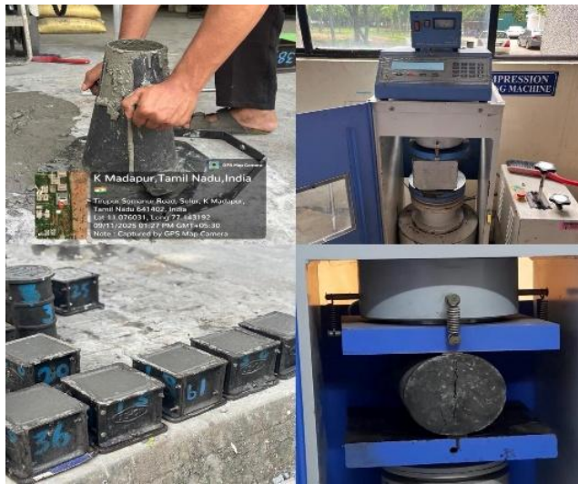
Fig. 1. Specimen preparation and compression testing process.
