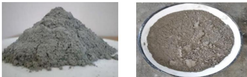
Fig. 1. Physical appearance of OPC and CDA used as a partial replacement of cement.
