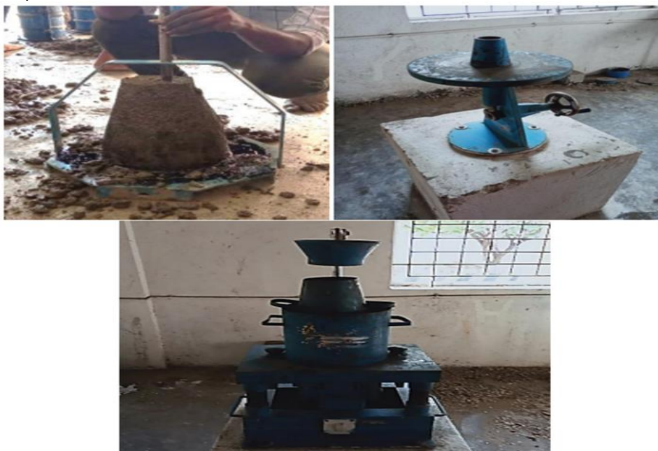
Fig. 3. Workability test on Concrete
