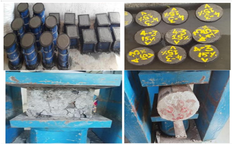
Fig. 4. Casting, Curing and Testing of Sample Specimen
