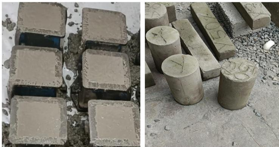
Fig. 2. Specimen casting (cube, cylinder and prism)
