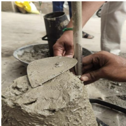
Fig. 3. Workability assessment by slump cone test
