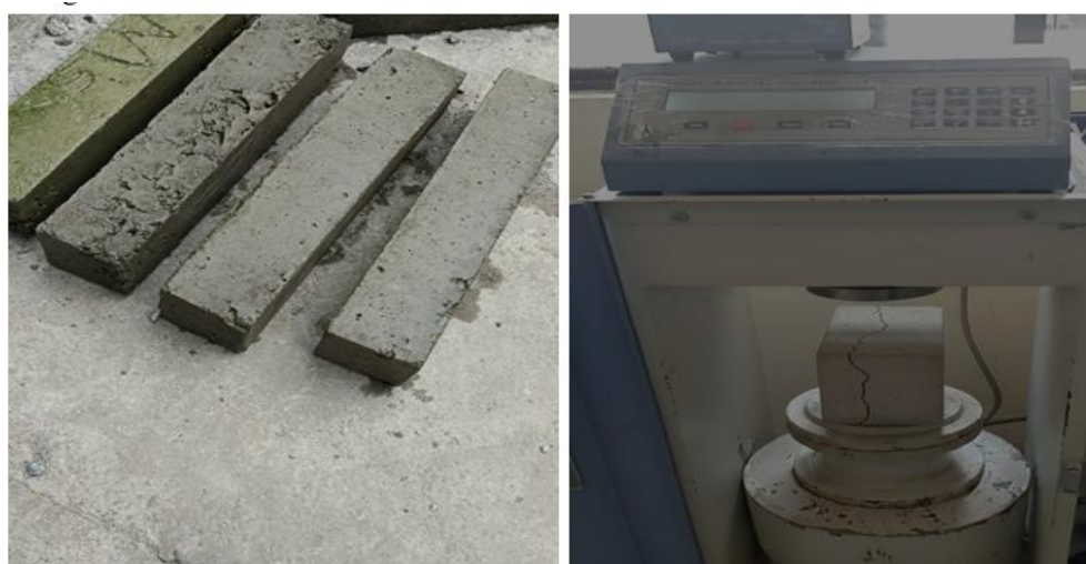
Fig. 6. Flexural strength test of concrete prism specimen
