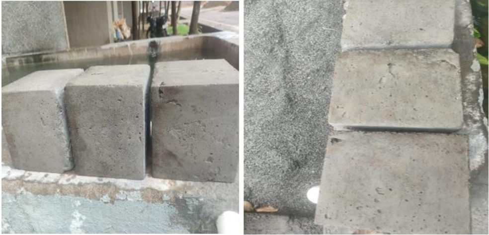
Fig. 8. Water absorption of concrete cubes
