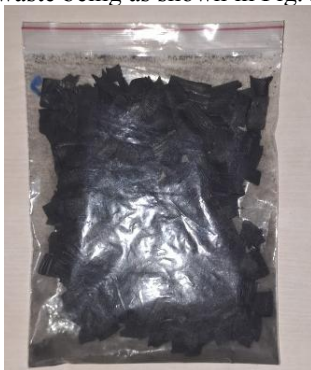
Fig. 2. Activated carbon produced from areca bat waste after activation
