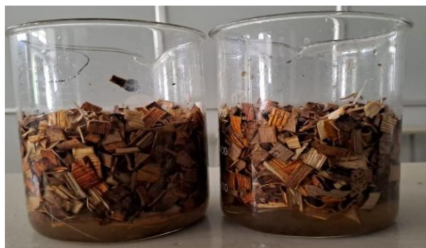
Fig. 1. Pre-treatment of chopped areca bat waste prior to activation
