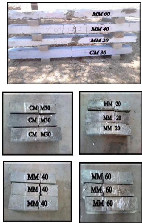
Fig.10. Flexural failure of RCC and PCC beams.
