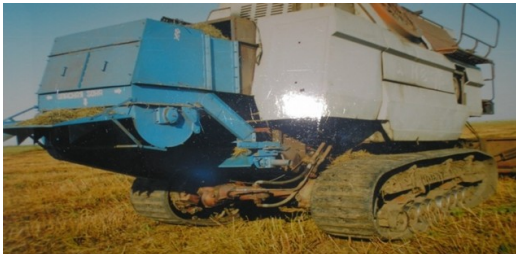
Fig. 3. Grinder - spreader - straw roller "IRVS-1200" in the aggregate with the grain harvester "SZK - 1200 RAG".
