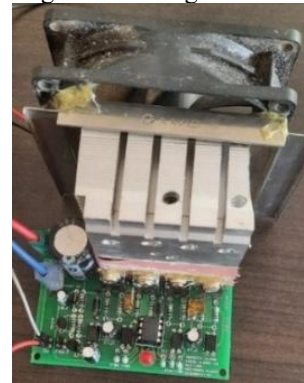
Fig. 5. Final Inverter PCB Assembly
