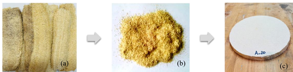
Fig. 1. Fabrication process of bio-based insulation panel derived from luffa materials: raw luffa sponges (a); fine fiber particles (b); final luffa panel (c).
