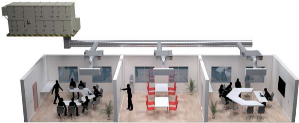
Fig. 6. Exemplificative non-exhaustive picture representing a possible solution of sensible heating and cooling of indoor building spaces by eliminating local in-room humidity condensation (and the related drain pans and drainage pathways) and by using calibrated humidity in air-renewal provided to each fan coil by a centralized air renewal and purification AHU [12]
