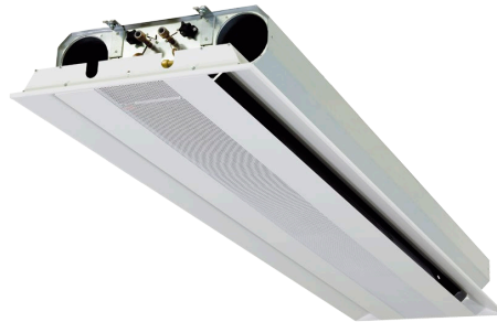
Fig. 8. Example of active type of chilled beam – Source: Roccheggiani S.p.A.: it can provide sensible heating and cooling controlling latent heat through calibrated humidity fresh air intake from centralized AHU. Normally designed for ceiling installation they use traditional tube and fin technology, without any kind of drain pan in room ambient.
