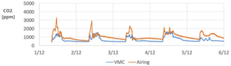
Figure 7. CO 2 (ppm) concentration during a school week. Comparison between a classroom with VMC and a classroom with airing (manual opening of windows) in Nereto (Teramo, TE)
