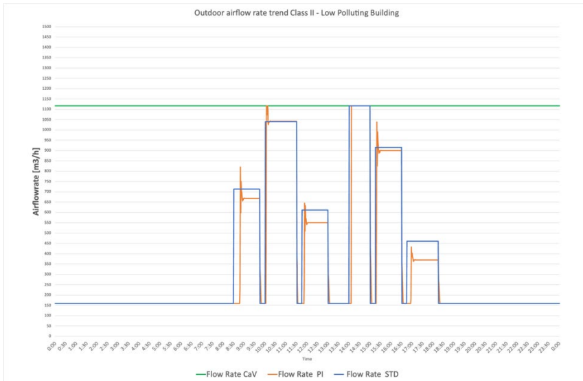
Fig. 2. Airflow profiles for the three control strategies applied to a system sized according to Class II – Low Polluting Building.
