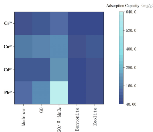
Figure 2. Adsorption capacity thermograms of heavy metal ions by different adsorbents.
