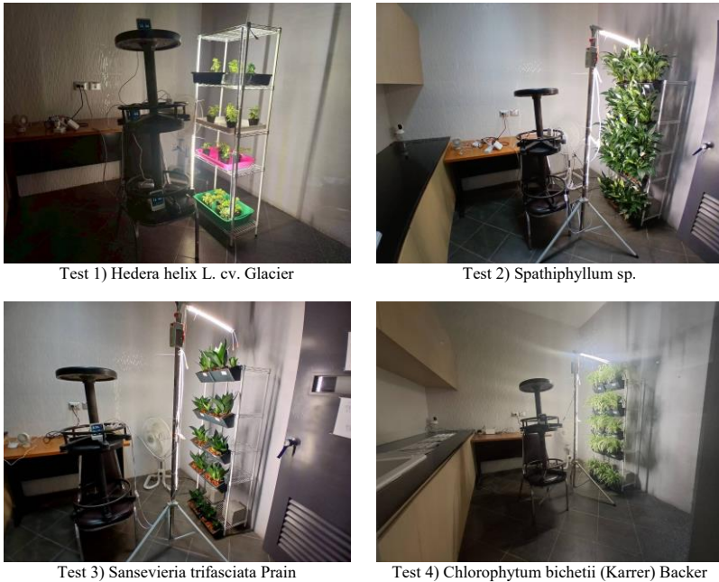
Fig. 2. Mock-up room test setups with ornamental plants to mitigate VOCs emissions in practical applications
