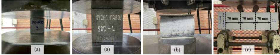
Fig. 2. Test results: (a) compressive strength, (b) splitting tensile strength and (c) flexural strength.
