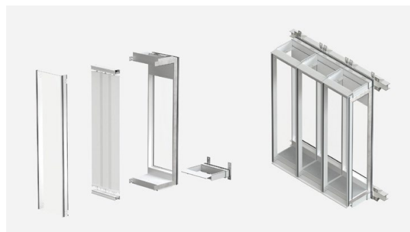
Fig. 1. Composition of cartridge facade
