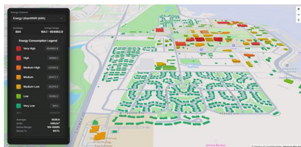
Fig. 5. Spatial distribution of simulated building energy consumption across 804 buildings in Mesa, Arizona for July 2025.
