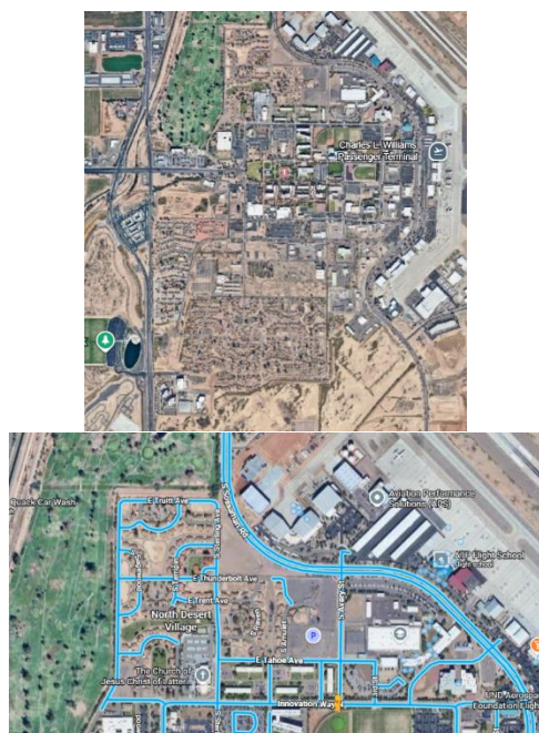
Fig. 1. Vehicle traverse route for mobile air-temperature measurements near ASU's North Desert Village in Mesa, Arizona.
