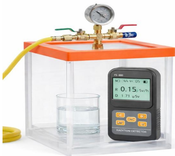
Fig. 1. Experimental setup for measuring background radiation emitted from a 150 ml rainwater sample using an FS-600 Geiger counter inside a vacuum chamber.
