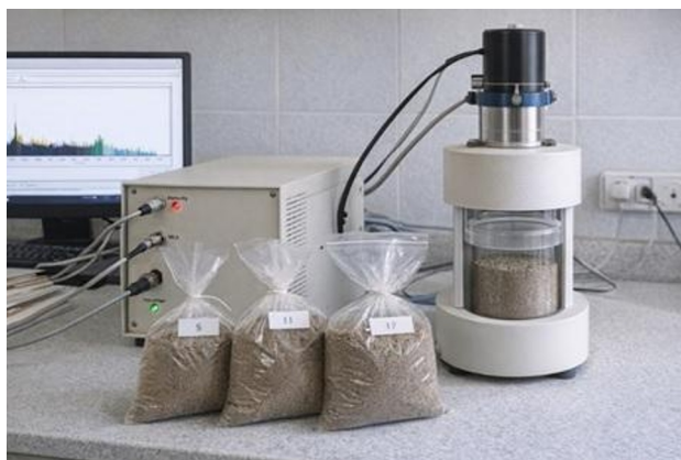
Fig. 2. NaI(Tl) detection system.
