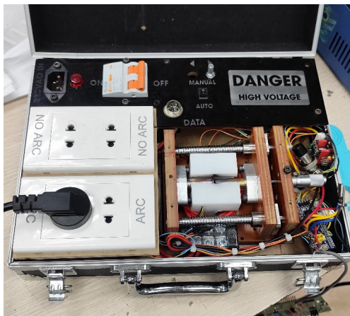
Figure 1: Experimental setup and data collection device for household arc fault measurements.
