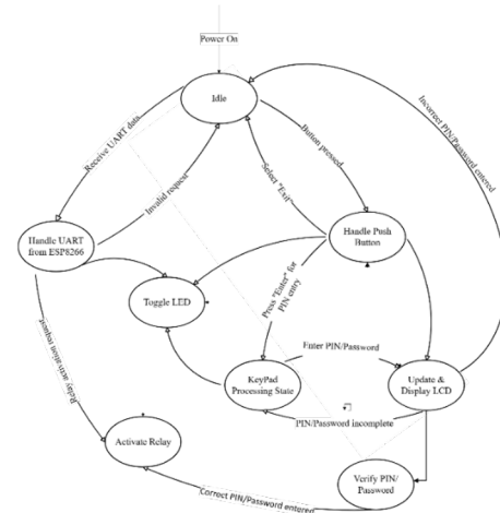
Figure 5. Finite-State Machine Diagram of ESP8266 in the Medicine Cabinet Controller
