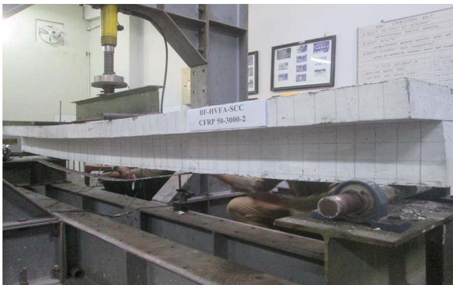
Fig. 10. Crack Pattern on Test Beam Specimen with CFRP Strengthening (BF-HVFA-SCC-CFRP50-3000-2)
