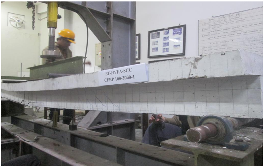
Fig. 7. Crack Pattern on Test Beam Specimen with CFRP Strengthening (BF-HVFA-SCC-CFRP100-3000-1)
