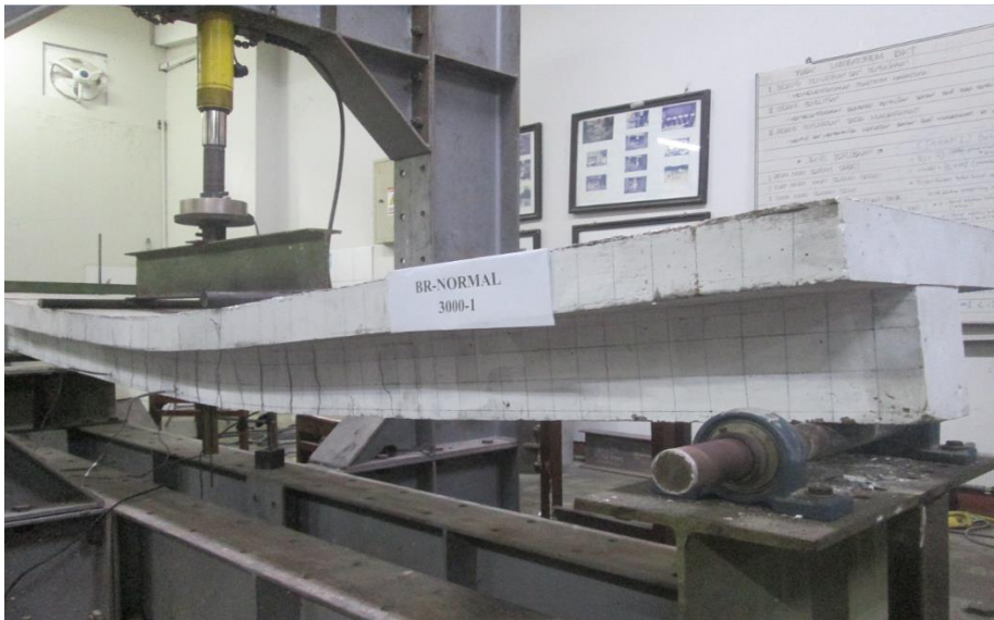
Fig. 6. Crack Pattern on Normal Test Beam Specimen (BR-Normal)
