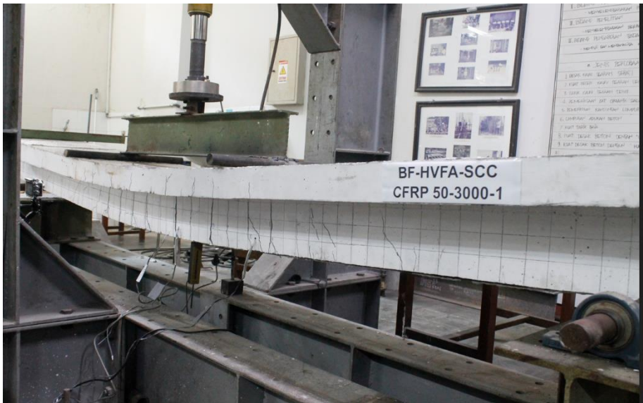
Fig. 9. Crack Pattern on Test Beam Specimen with CFRP Strengthening (BF-HVFA-SCC-CFRP50-3000-1)
