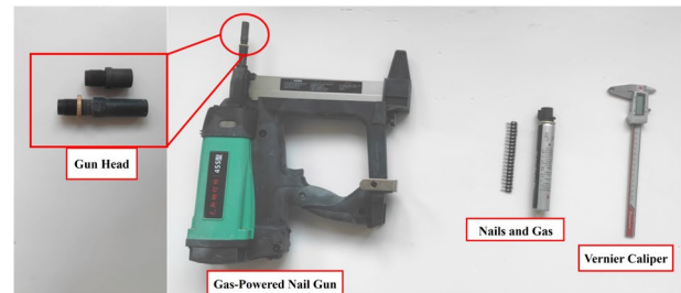
Fig. 8. Nail shooting test equipment
