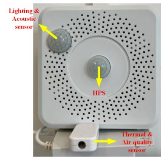
Fig. 3. A all-in-one IEQ sensor.
