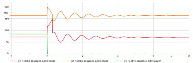
Fig. 13. Active power profiles of all generators following generator 3 trip and subsequent loadshedding.
