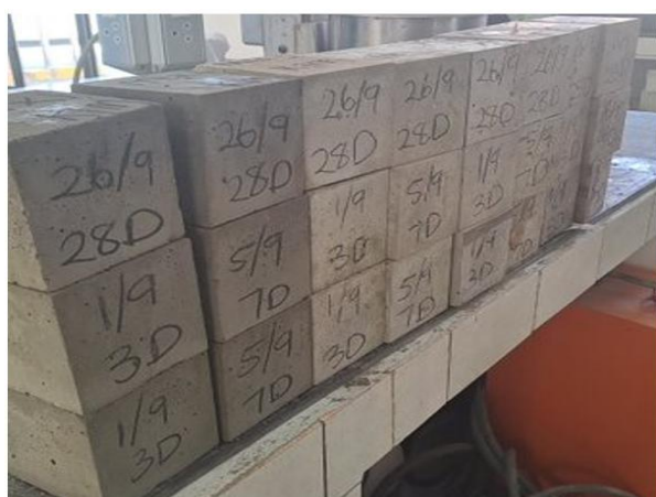
Fig. 1. Concrete cubes for compressive strength test
