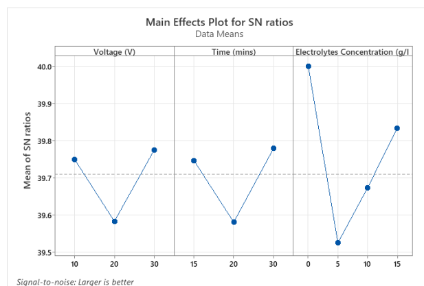
Fig. 6. Main effects plot for Signal-to-Noise ratios for Turbidity
