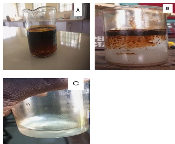
Fig. 11. Change in Colour of Crude Oil-Contaminated water. (a) Untreated water (b) Water during EC treatment (c) Water filtered after EC treatment
