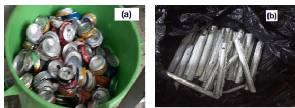
Fig. 2. (a) Waste Beverage Cans. (b) Fabricated aluminium anodes
