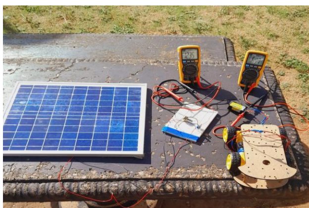
Fig. 14. Charging an EV battery with solar PV
