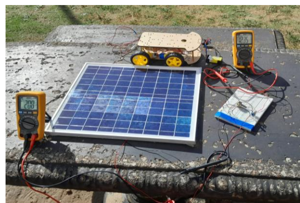
Fig. 15. Multimeters displaying an input voltage for a DC converter and output voltage
