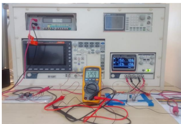
Fig. 13. DC converters for 18V to 12V and 12V to 9V after testing.
