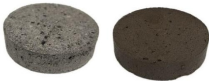
Fig. 1. Specimen prepared with dried peat (left, RUB 1) and moist peat (right, RUB m 1).
